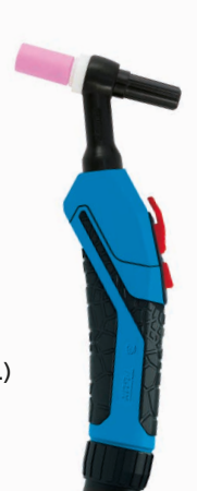
TBi SR 21 100% (10 min.) AC: 240 A DC: 340 A Ø 0.5-3.2 mm
