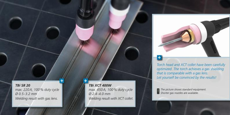
The TBi XCT collet creates a large area of contact between the electrode and the water-cooled torch head. This ensures an exceptionally efficient transfer of current and heat.
